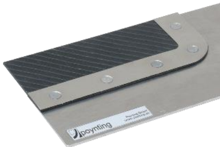
Figure 1: A carbon fibre reinforced composite (CFRP) sheet joint by means of EMR process with an aluminium sheet
