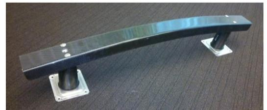
Hybrid bumper consisting of aluminium and carbon fibre reinforced composites
