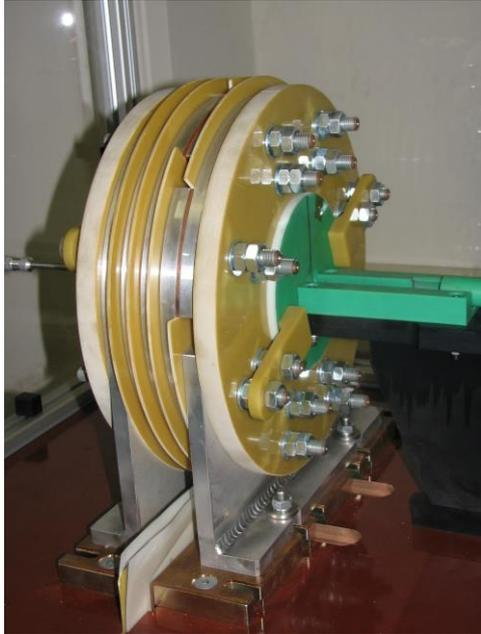
Tool coil used for electromagnetic joining
